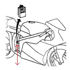
It must be installed not higher than 60 cm from the ground surface.
