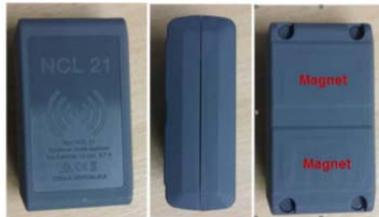
NCL21 unit is started during roadbook issuing before starting of reconnaissance. For whole reconnaissance the unit is working on its own battery. It is not necessary to plug the unit to any power supply.
